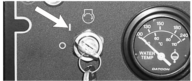
Figure 11.3 - Start Switch, Ground
