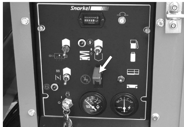
Figure 9.2 - Ground Control Box Emergency Stop Switch
