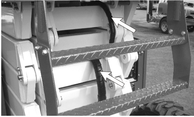
Figure 7.11 - Wiring Harness in the Scissor Stack
