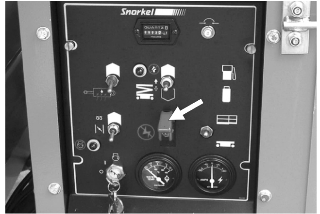
Figure 2.2 - Ground Control Box Emergency Stop Switch
