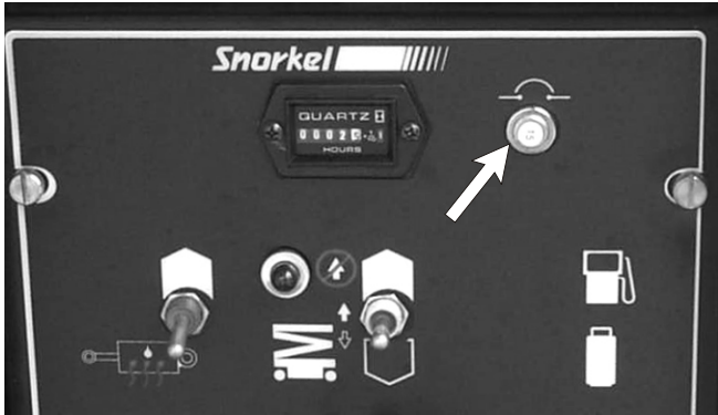
Figure 5.4 - Main Circuit Breaker
