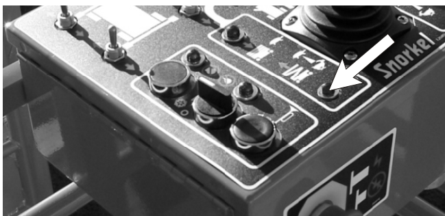
Figure 2.4 - Platform Overload Light
