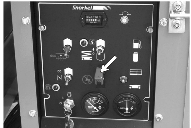
Figure 8.1 - Emergency Stop Switch at Ground Control Box
