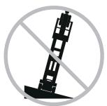
Models with outriggers: Do not lower the outriggers unless the machine is on a firm surface. Avoid drop-offs, holes, unstable or slippery surfaces and other possible hazardous conditions.
