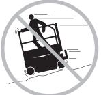
Limit travel speed according to condition of ground surface, congestion, slope, location of personnel, and any other factors which may cause collision.
